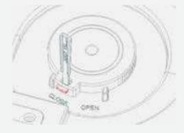
Remove the UV lamp from its packaging and insert it carefully. Then rotate clockwise until it clicks and locks.
