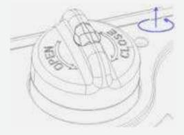
Remove the new MAXI filter from its packaging and insert it. Then turn clockwise to install.
