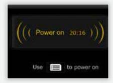
Touch the key to confirm you want it to turn on. When your BIBO switches back on from the 'Power on/off' mode, the hot tank will take approximately 5 minutes to heat back up to the maximum temperature and the cold tank will take approximately 15 minutes to chill back down to the minimum temperature.
