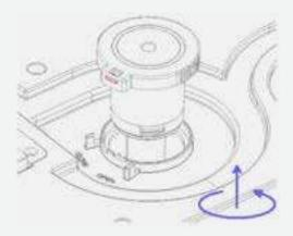
Once the UV lamp has been replaced, select 'Replacement' from the menu, select 'UV' and touch the replacement. The counter will be reset to '360 days left'.
