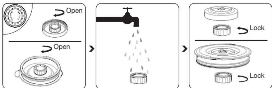
Turn over the lid (3) and open the backflow prevention cap by turning it anti-clockwise to remove it from the lid (3).
