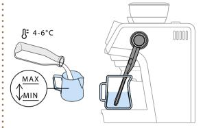
Fill the milk jug with the volume of milk you'd like in your coffee, without exceeding the maximum line. Place the steam wand into the milk jug and rest the milk jug onto the milk jug area as shown in the picture. In the correct position, the dial at the top of the steam wand should be in position 'A'.
