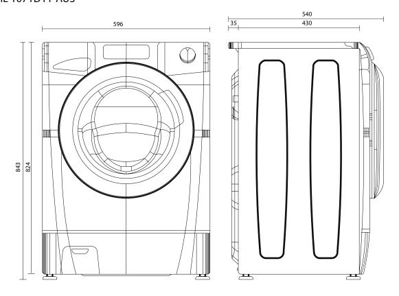
Model 31007835 Freestanding 7kg washing machine Max absorbed power (kW) 1500 Voltage V 220-240 Length inlet hose 150cm, length drain hose 200cm, length electrical supply cord 160cm
