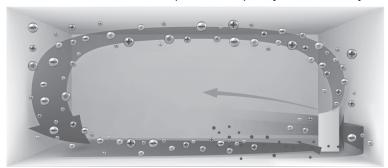
Faster airflow at a 20° angle collects dust at lower levels in the room for more effective cleaning.
