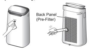
Remove the dust gently with a cleaning tool such as a vacuum cleaner.
