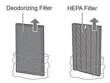
3. Install the filters in the correct order as shown.
