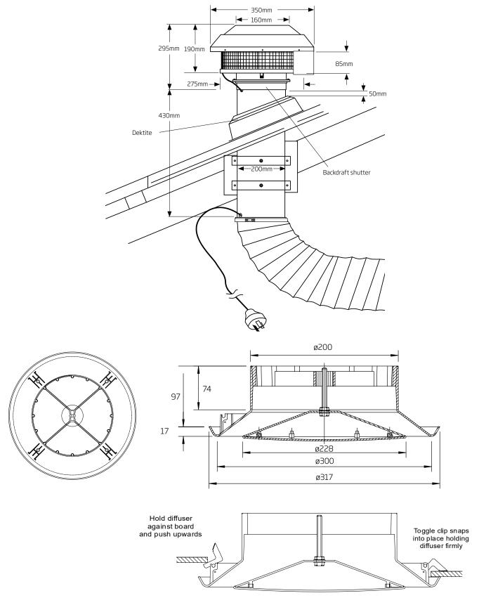
The cone in the middle can be adjusted to increase or reduce airflow by winding anti-clockwise or clockwise
