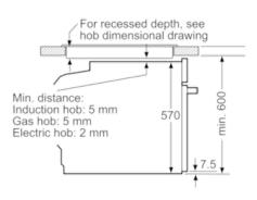
measurements in mm
