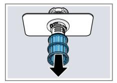
**4.** Press the locking catches ① together and lift the coarse filter out
