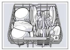
Cutlery basket a1 Large plates up to a diameter of 34 cm can be arranged in the bottom basket as shown.
