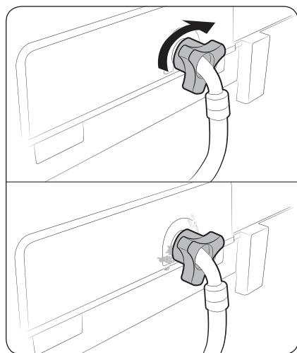
3. Reinsert the filter. Make sure it is tightened against water leaks.
