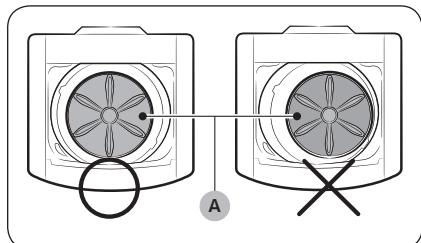
See if the washing machine is level by checking the position of the tub:
