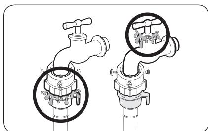
8. Open the water tap and check if there are any leaks around the connection areas.
