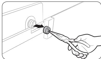
1. Use pliers to pull out the mesh filter from inside the water inlet as shown.
