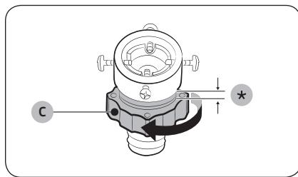
3. Hold the adaptor and turn **part (C)** in the arrow direction to loosen it by 5 mm (\*).
