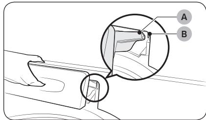
5. Return the **Bubble Kit (A)** to the detergent compartment. Replace the drawer by placing the **drawer rail (A)** on the **compartment rail (B)** while tilting the drawer downward.
