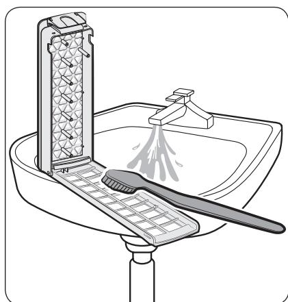
2. Unlock the cover, and clean the filter with running water and a brush.
