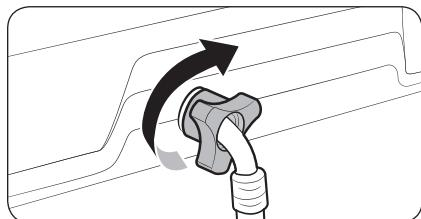
7. Connect the other end of the water hose to the inlet valve on the back of the washing machine. Turn the hose clockwise to tighten.
