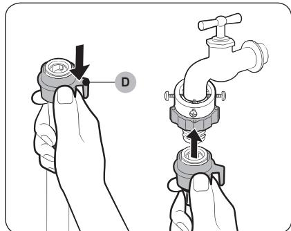
6. While holding down **part (D)**, connect the water hose to the adaptor. Then, release **part (D)**. The hose fits into the adaptor with a clicking sound.
