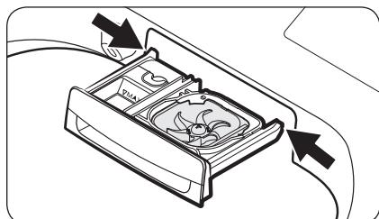
2. To remove, pull the detergent drawer while pushing the ends of each side.
