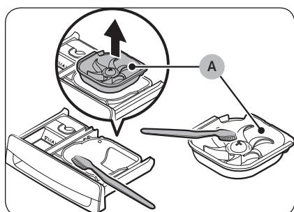
3. Remove the **Bubble Kit (A)** from the compartments. Rinse the **Bubble Kit (A)** and the drawer in warm water and clean with a soft brush.
