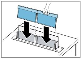
To avoid causing damage, do not bend the grease filters.
