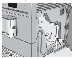
■ Press and hold the button under the brew unit handle ① and, whilst doing so, turn the handle to the left ②. ■ Carefully pull the brew unit out of the coffee machine.
