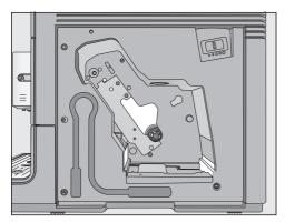
Clean the interior of the coffee machine. Make sure that the areas highlighted (in white) in the illustration are cleaned especially well.
