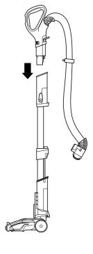
1 Place motorized floor nozzle on floor and insert wand.
