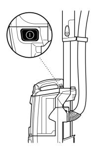
2 The Powered Lift-Away DuoClean™ has a 2-speed Slider Switch on the handle. Move the Slider Switch to appropriate speed setting. The soft roller spins in both settings to pick up extra dust and debris.
