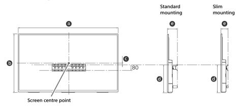
Unit: mm Screen **Display dimensions** centre Length for mounting dimension **Model Name** a 0 G 0 e Standard Slim mounting mounting KD-55X7500F 1,242 721 95 460 142 100 KD-49X7500F 1,101 645 15 314 120 78 970 571 120 78 KD-43X7500F 23 315
