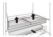
1 Press the levers on either side of the drawer support.
