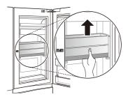
2 To lower the Adjustable Moving Basket, press up to release the levers at the bottom of the basket and lower the basket until it clicks into place.
