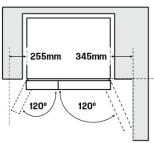
When positioned in a corner area, spacing of at least 345mm on the right hinge side and 255mm on the left hinge side will allow the doors to open enough to enable the removal of bins and shelves.
