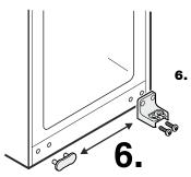
6. Transfer lower hinge bracket and cover plate to the opposite side.
