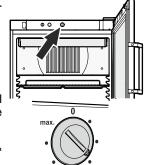
The nearer the temperature control is to the **max**. setting, the colder the interior temperature.
