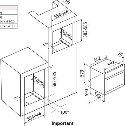
\*100mm WIDE SUPPORT EACH SIDE WITH 50mm CLEARANCE UNDERNEATH
