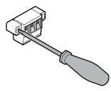
Remove the terminating resistors from the appliances in between.
