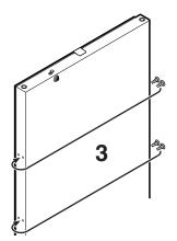
4. Transfer pin on hinge bracket to the opposite side.
