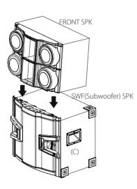
3. FOOT (A) of FRONT SPK is mounted on the top of the guide hole (B) of SWF(Subwoofer) SPK.
