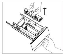
Flush it out under a tap to remove any traces of accumulated powder.
