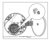
Make sure that the impeller of the pump can turn. If this does not occur, contact the service centre.
