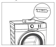
If you do not have a spirit level, as a guide use the edge of a door frame, cupboard or bench to check that the washing machine is leveled.
