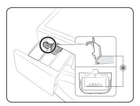
First insert the provided liquid container in the II main-wash compartment. Then, apply liquid detergent to the container below the marked max line (A).
