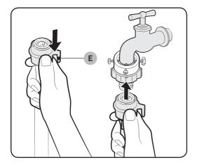
**6.** While holding down part (E), connect the water hose to the adaptor. Then, release part (E). The hose fits into the adaptor with a clicking sound.
