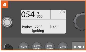
Once the probe alarm is set, the home screen will display the grill temperature, goal probe temperature, and grill status. A tone will sound when your meat reaches the set alarm temperature. If using the Traeger WiFIRE® app, you will receive a push notification on your connected smart device, along with a display of your grill's status throughout the cooking process.
