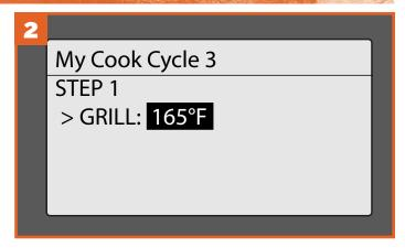
At Step I, a prompt will display to select a grill temperature (default temperature is I65°F [74°C]). Turn the Selection dial to the desired temperature and press the center of the dial to select.
