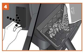
Once the hopper's empty, close the door, replace the fastener, and refill the hopper with a different flavor of TRAEGER® BRAND HARDWOOD PELLETS.
