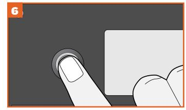
Turn off the grill by pressing and holding the Standby button for 3 seconds, initiating the shutdown cycle. When the full shutdown cycle finishes, seasoning of your grill is complete.
