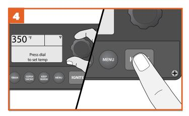
The home screen will display "Press dial to set temp." Turn the Selection dial clockwise to 350°F (I77°C). Press IGNITE, close grill door, and run grill for 20 minutes once it has reached the set temperature.
