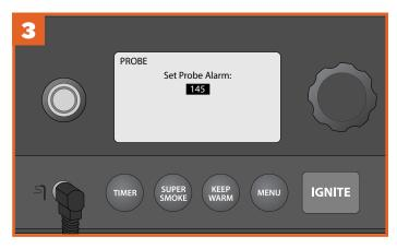
Rotate the dial to the desired food temperature. Press the dial center to select/confirm.
