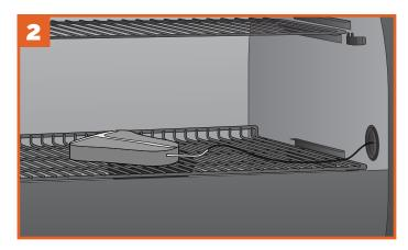
Once the grill is preheated to the desired temperature, load food into the grill. Feed the probe through the grommet on the side of the grill and insert the probe tip halfway into the thickest part of the meat—not in the fatty portion or touching bone.
