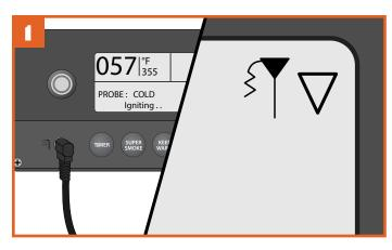
Plug the probe into the probe jack located on the WiFIRE® Controller. See "Using Your Grill" to turn on the grill. Once the grill is on, the controller will recognize the probe and the probe icon will light in the controller screen's upper-right corner.
