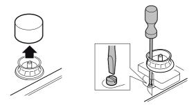
**Never remove the valve reinforcing ring.** The valve reinforcing rings guarantee the watertightness of the appliance's interior from liquids and dirt, which might otherwise prevent its correct operation.
