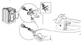
**4.** Insert the mesh filter again. Connect the inlet hose to water tap and washing machine again. Do not use a tool to connect the inlet hose. Open the water tap and check that all connections are tight.
