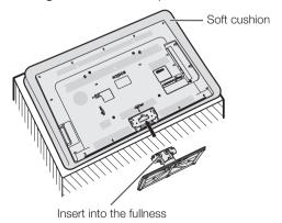
Insert and tighten middle screws into the holes on the rear of the TV.
