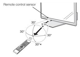
\* When mounting the TV on the wall.
