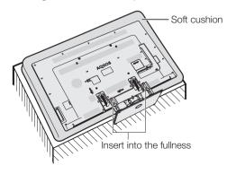
Insert and tighten middle screws into the holes on the rear of the TV.
