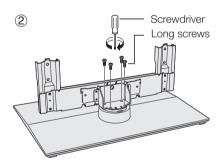
Insert the stand into the openings on the bottom of the TV (hold the stand so it will not drop from the edge of the base area).
