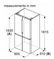
Front is adjustable from 1830 to 1847, with front levelling feet fully extended
