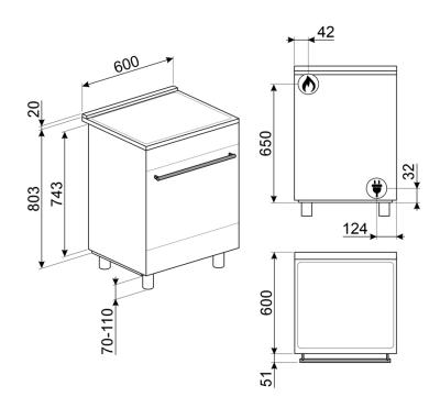
**Dimensions**  $600 \text{mmW} \times 873 \text{-} 913 \text{mmH} \times 600 \text{mmD}$
