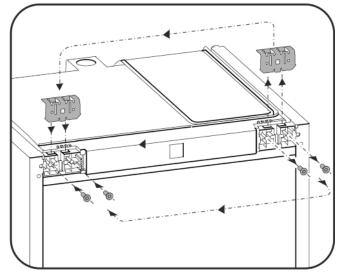
► Move the fixing bracket to the opposite side.
