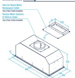
Transition Duct - X1DK.TRANS Included with Ultra On-Board Top Duct Configuration
