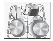
It is suggested that large items, and items that are most difficult to clean, are placed in the lower basket — eg pots, pans, lids, serving dishes etc. It is preferable to place serving dishes and lids on the side of the racks to avoid blocking rotation of the top spray arm.
