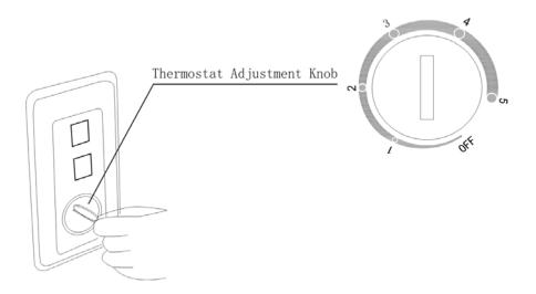
The temperature of the freezer is adjusted by turning the knob assembled on the thermostat.
