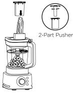
**6a** Add the prepped ingredients you want to slice, shred, or grate through the feed chute on the lid. Use the 2-part food pusher to help guide the food through the feed chute. The middle piece of the food pusher is removable to use for narrow ingredients. **DO NOT** process ingredients past the **DISC MAX** line on the pitcher.
