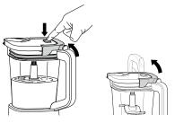
8 Remove the lid and dough blade assembly before removing contents. To remove the lid, press the release button above the handle, and rotate the lid tab counterclockwise out of the lock position, then lift the entire lid up.
