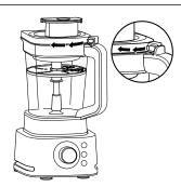
4 To install the feed chute lid on the pitcher, place the lid tab to the right of the handle. Press the lid down until it is secure. Rotate the tab clockwise until it clicks into place on the pitcher handle. Once the lid is locked in place, press the Power button to turn unit on.
