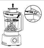
8 To remove the lid from the pitcher, press the release button above the pitcher handle, and rotate the lid tab counterclockwise out of the lock position, then lift the entire lid up.
