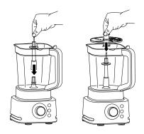
3 Place the disc spindle onto the drive gear inside the pitcher. Then, use the plastic grip to grasp the disc and place it over the spindle.
