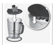
2. Put the ingredients in the blender jug. Do not exceed the maximum level as indicated on the jug. Align the two fasteners of the blender lid with the two clip positions of the blender jug and push down to lock in place "Click".
