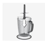
Place the blender jug on a flat surface. Make sure that the non-slip ring is properly placed. Fit the blender blade over the spigot inside the blender jug. Caution: The blades are very sharp!
