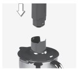
3. Insert the motor unit into the opening of the lid and lock into position. Plug into the power outlet, select the speed and press the power button to start. Release to stop. Remove the motor unit by pressing the release button.
