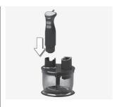
3. Insert the motor unit into the opening of the lid and lock into position.
