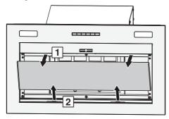
► Fold down the metal grease filters 1 at the front and carefully remove from the slots 2 in the fixture.
