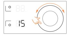
**2.** For setting and adjusting the power level, rotating the magnetic knob.
