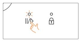
2. Touch the Pause | |/ |> sensor for 3 seconds within 10 seconds after Power On.
