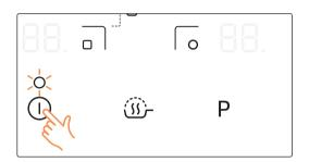
To completely switch off the appliance, use the **On/Off control** ① sensor.
