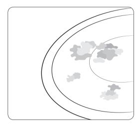
Remove burnt-on sugar, melted plastic, aluminium foil or other materials with a glass scraper immediately and while still hot.
