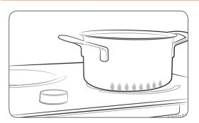
Virtual flame technology creates the appearance of flames when you turn on an induction element.
