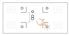
After switched on, press the corresponding cooking zone to activate the flash signal for the corresponding cooking zone display.
