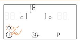
The appliance is switched on using the **On/ Off control** ① sensor.
