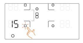
To switch off a cooking zone, press the cooking zone selector during 2 seconds.
