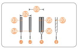
2N~ (16A): Separate the 2-phase wires (L1 and L2) before connection.
