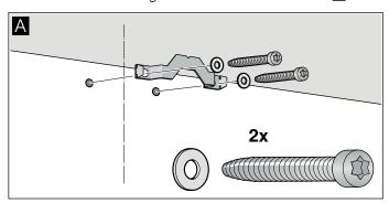
2. Screw on brackets for the extractor hood hand-tight. Do not firmly tighten the screws. **B**
