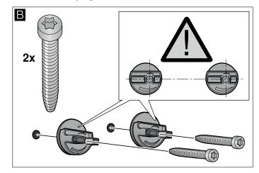
Screw in the threaded bolt, leaving it protruding out of the wall by 5–9 mm.
