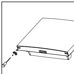
Use a flat-bladed screwdriver to pry open the upper door sleeve and corner plastic cover. Turn the door sleeve 180° then put it back on the upper door. Turn the plastic cover 180° then put it to opposite side where the top hinge bracket will be fixed.
