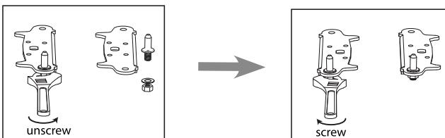
5. Refit the bracket fitting the bottom hinge pin. Replace both adjustable feet. Transfer the lower door to the property position.
