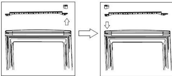
8. Install the upper door, fix the upper door hinge onto the cabinet.
