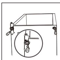
6. Make the middle hinge reverse the direction 180°C, then transfer it to the left property position. Make the middle hinge pin in the upper hole of the lower door, then tight the screws.
