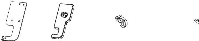
1. Close upper door, take out the screw from the top hinge covers by cross screwdriver. Take off hinge cover, then unscrew top hinge and take off upper door.
