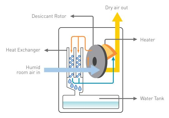
Desiccant rotor dehumidifiers use a desiccant (a substance that adsorbs water in a vapour state) that is mounted on a rotating wheel (called a rotor). In the Ionmax ION612 and ION632, the desiccant material used is Zeolite.
