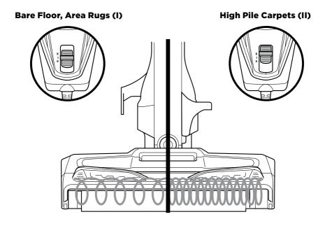
The Shark® Rocket® Complete with DuoClean $^{\text{\tiny M}}$  has a 2-speed power slider switch on the handle. Slide the power switch to appropriate speed setting (I or II) and start cleaning.
