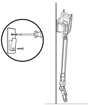
**2** Use the wall mount that is included. Drill two 8mm holes into the wall and insert the provided plastic anchors into the holes. Using a Phillips-head screwdriver, screw the wall mount into the plastic anchors. Hook the catch on the bottom of the handheld vacuum onto wall mount.
