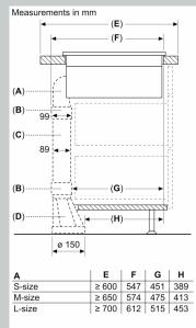
A: 90° Bow B: Connector sleeve C: Straight tube D: Straight adapter round-flat
