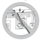
If the speaker cable core comes into contact with any metal portion of the receiver's body, it may damage the speakers and cause smoke and fire.
