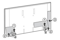
2 Remove the screws from the rear of the TV.
