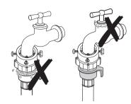
If the water tap has a screw type tap, connect the water supply hose to the tap as shown.
