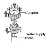
2. First, using a '+' type screwdriver, loosen the four screws on the adaptor. Next, take the adaptor and turn part (2) following the arrow until there is a 5 mm gap.
