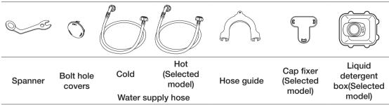
\* Bolt hole covers: The number of bolt hole covers depends on the model (3~5 covers).
